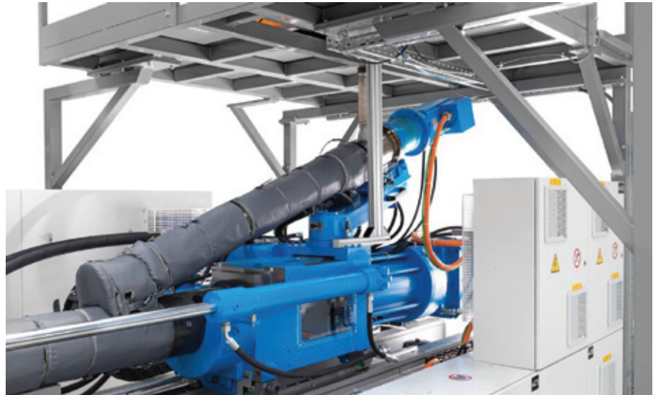
The DCIM process from KraussMaffei uses a single-screw extruder
